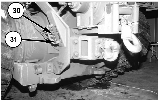
Remote Charging Valves (Left Side Shown, Right Side Symmetrical). (30) Charging valve. (31) Charging valve.
