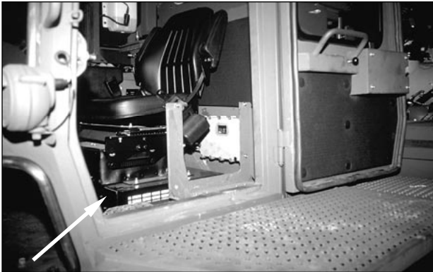
Air-Conditioning Unit, Under Operator's Seat.
