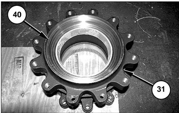
148. Install Duo-Cone Seal (40) into hub (31), using Tooling (E). Refer to “Duo-Cone Seals” in this module.
