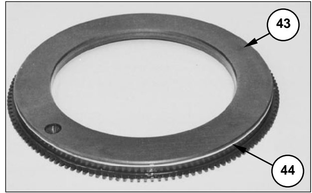
38. Remove ring (44) from piston (43).
