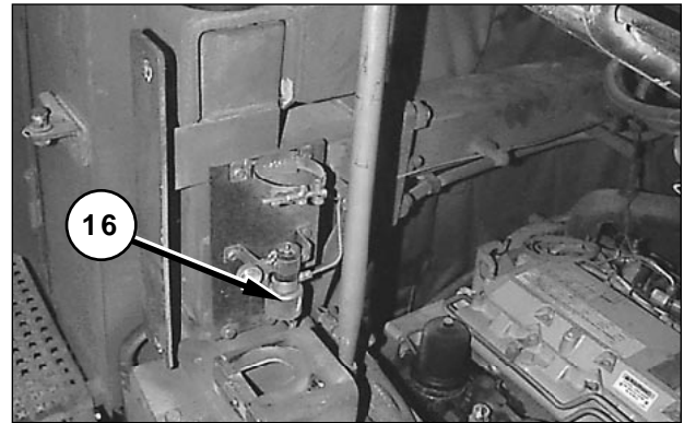
Engine Compartment. (16) Ether injection solenoid.
