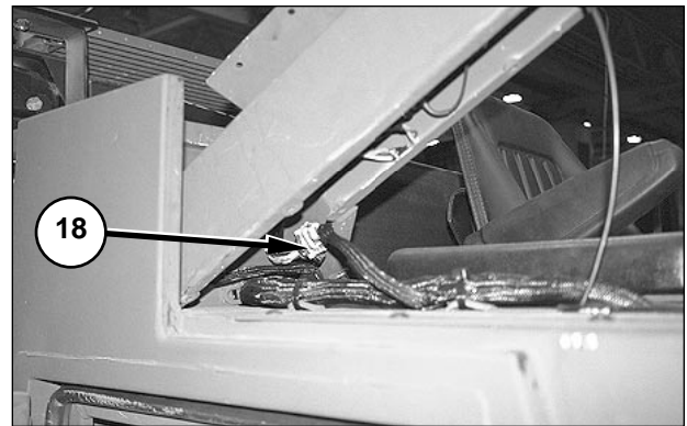
11. Disconnect connector C113 (18).
