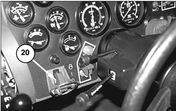
Instrument Panel. (20) Start switch.
